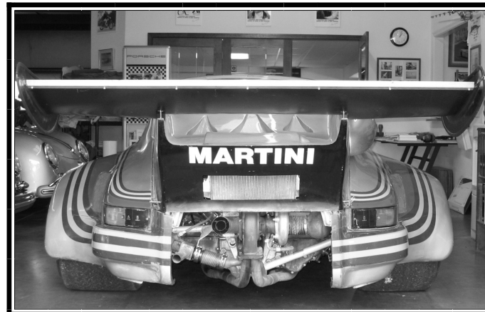
wider than it is long! This 1974 911 RSR 2.1 liter is the first turbocharged 911 racecar and is the prototype for the highly successful 935. It produced 480 horsepower at 8000 rpm. Photos by Phil Audibert
