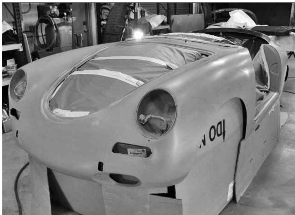
PRIMED OUT AND READY TO PAINT.
