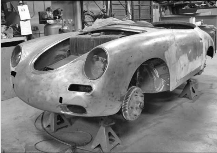
Left Front, Door in Place, Old Paint Being Removed
